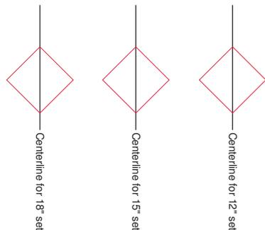
Do not cut the template for use in an 18" wide cabinet opening
