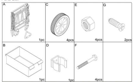
Assembly: please <u>use tools</u> such as screwdrivers, wrenches, pliers to tighten the screws. it comes off easily if you tighten it by hand only.
