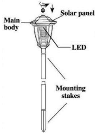
**Stake:** Connect mounting stakes together by applying pressure. Then, screw counter clockwise the tip to the main body. Now, your light is ready to go into the ground.
