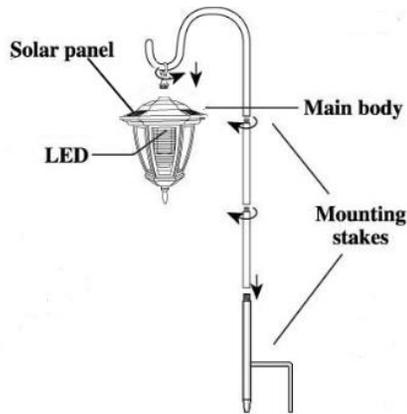
**Hanging:** Connect hanging hook to mounting stake by screwing clockwise. Then, repeat action with another mounting stake. Finally, connect assembled mounting stakes to "H" stake by applying pressure. Then screw counter clockwise the hook into the main body topper
