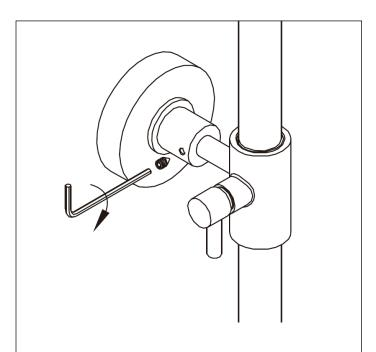
**11.** Slide the shower set into the mounting bracket and secure into place with the set screw.
