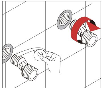
**2.** Connect the installation adapters to the water supplies. Use a small amount of teflon tape to ensure a watertight seal.
