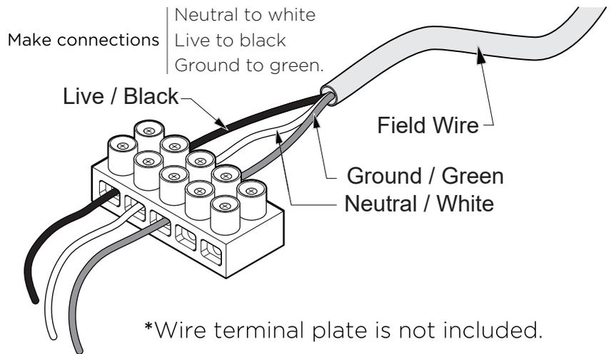
**Electric wiring:** Be sure to provide enough wire to make the proper and safe connection to the Field/Power.
