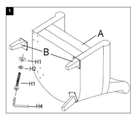
Attach front leg(B) to seat (A), using Allen bolt L(H1), flat washer (H3), and Spring washer (H2), Tighten with allen key (H4)
