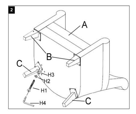
Attach rear leg(C) to seat (A), using Allen bolt L(H1), flat washer (H3), and Spring washer (H2), Tighten with allen key (H4)
