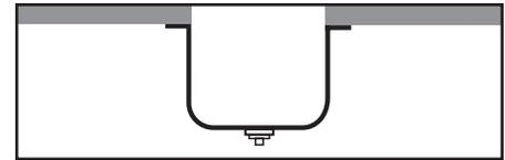
**Negative Reveal** – The countertop extends over the edge of the sink on all sides by approximately 1/8". Use caution with this installation to be sure that accessories such as colanders or cutting boards will fit properly.
