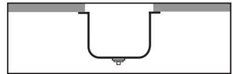
**Zero Reveal** – The countertop meets the edge of the sink, fitting flush with the sink bowls.
