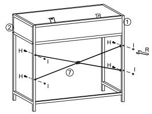
Use screw and nut(H/I) to fix back X bar(7) to left and right legs(1,2).
