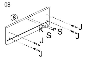
Screw 4pc cam lock pin(J) on drawer front panel(8), use 2pc screw(S) to fix handle(K) on (8).
