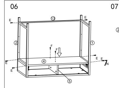
Use 2pc screws(F) to fix bottom panel(4) on middle divider panel(5), use screw(E) to fix left and right legs(1,2) to bottom panel and metal tube(13).
