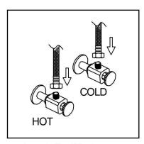
5. Attach flexible hose to water supply.
