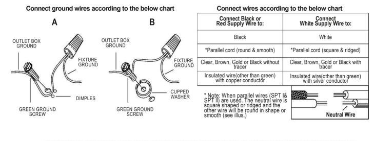
Twist wires together with plastic wire connectors (D) until tightly joined, and wrap each connector with approved electrical tape for a more secure connection, then carefully tuck all wires into the outlet box.
