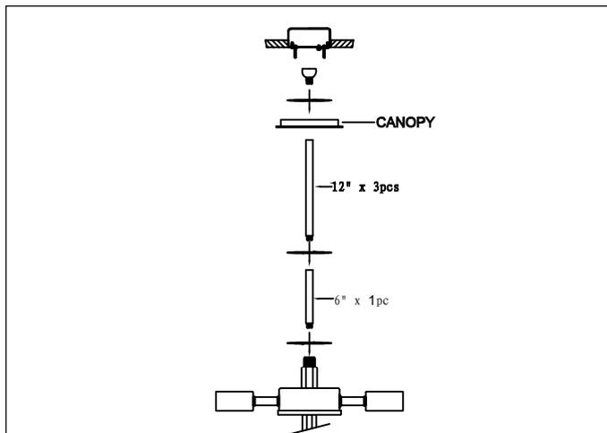
1. Remove mounting bracket from fixture and install to electrical box
