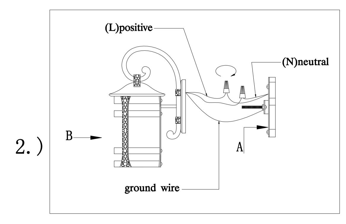
Step.2: Attach back plate to mounting bracket and tighten ball nuts so fixture meets wall. Caulk fixture where back plate meets the wall with silicone sealant.
