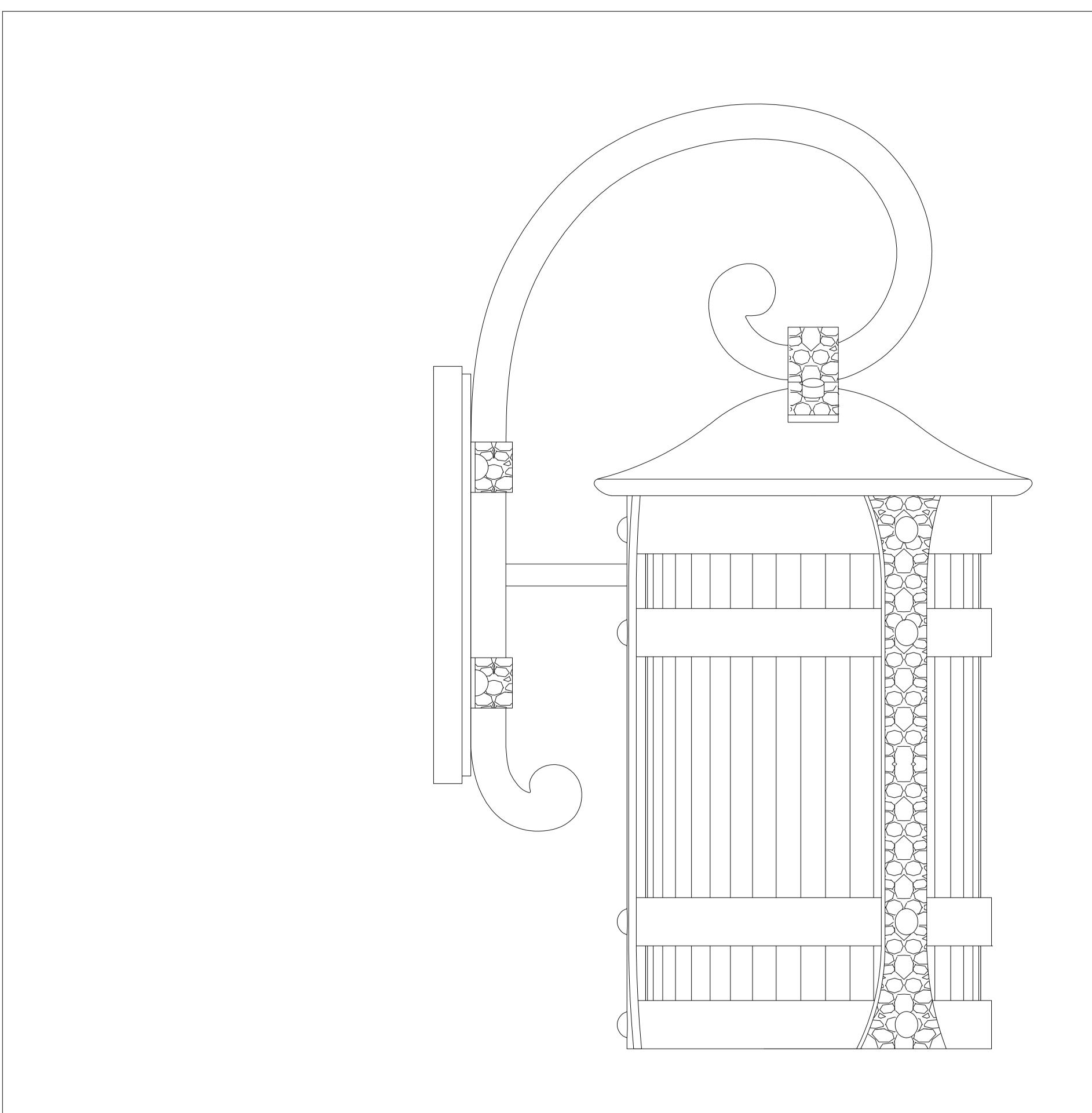
To prevent water intrusion, caulk around back-plate where fixture meets the wall using outdoor silicone sealant. Leave a small gap at the bottom to allow moisture to exit.
