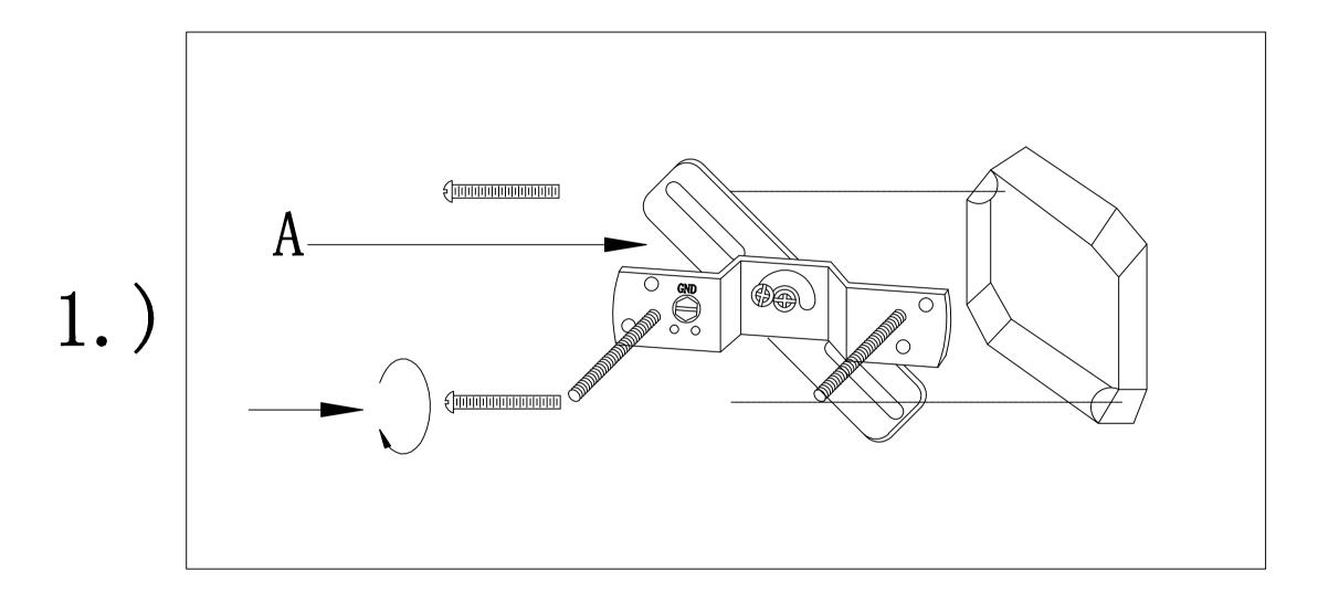
Step.1: Remove mounting bracket from fixture(B) and install to electrical box. then wire fixture to wires in outlet box. Copper wire is for Ground.
