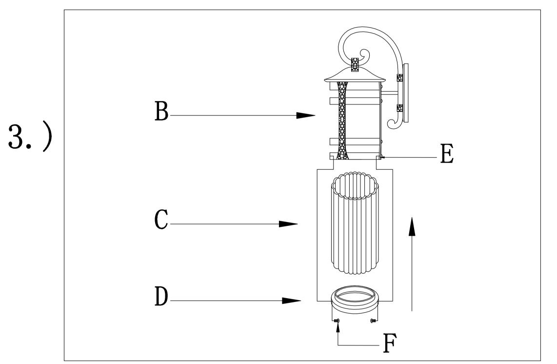
Step.3: Attach glass(C) and secure using bottom plate(D) to the fixture using screws(F) at point(E).
