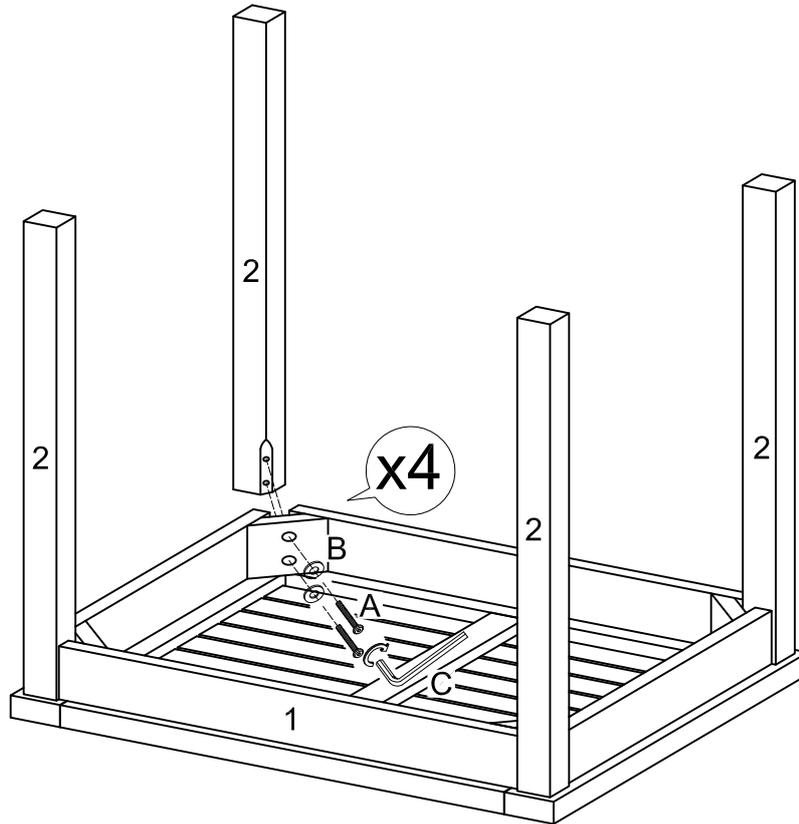
Use wrench (C) to secure top frame (1) to leg (2) with bolt (A), and washer (B).
