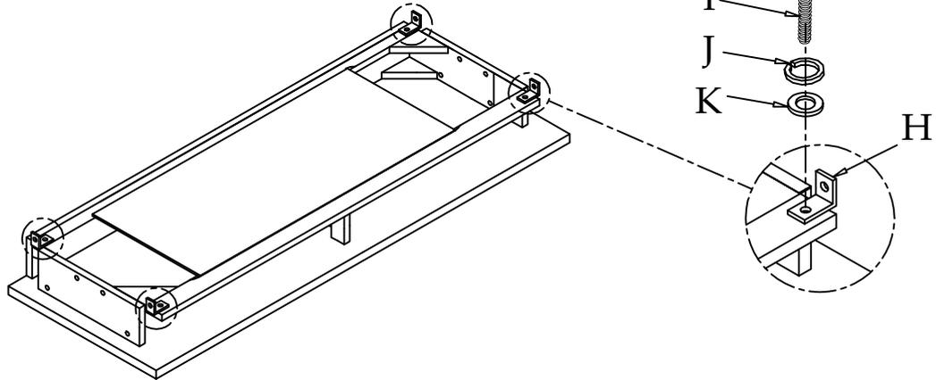
Step 3 : Using the Allen key to tighten all bolts
