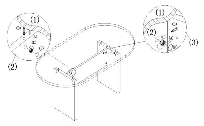
Attension: Please apply Part (P) Cam Covers over each exposed Part (C) Cam Lock after finishing the installation.
