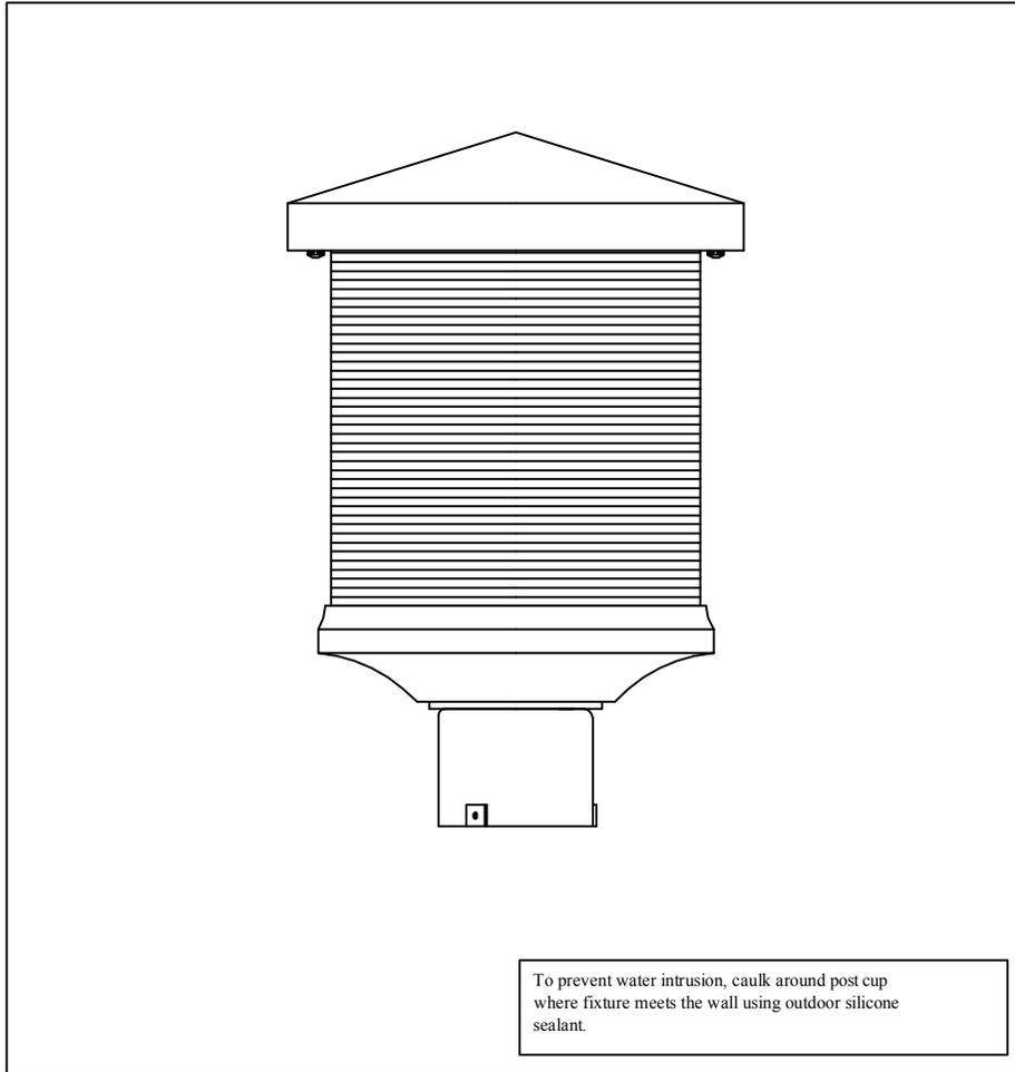
To prevent water intrusion, caulk around post cup where fixture meets the wall using outdoor silicone sealant.
