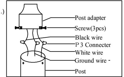
Step.1: Wire fixture to supply circuit in the post mount.
