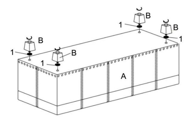
Place the Ottoman (A) on its back on a flat smooth surface. Attach Ottoman Feet (B) to Ottoman (A) with Washers (1) to each corner.
