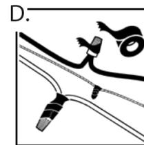
**D.** Attach wire nuts. Tape nuts and wire together.
