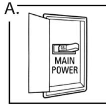
**A.** Shut off main power at the circuit breaker or fuse panel before removing old fixture.
