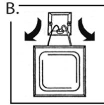
**B.** Remove old fixture. Disconnect wiring.
