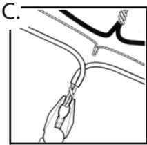
**C.** Strip 1/2" of insulation from wire ends. Twist stripped ends together with pliers. Connect fixture Hot wire to house Hot wire, fixture Neutral wire to house Neutral wire and fixture Ground to house Ground wire.
