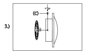
Step.3: Install fixture to bracket and tighten finials (C) at the ends of the canopy to secure.
