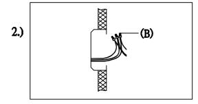
Step.2: Wire fixture to wires (B) in outlet box. Copper wire is for Ground.
