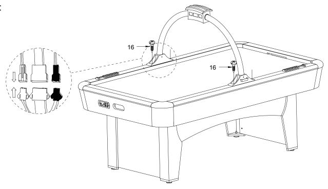
Attach scoring unit to table, being careful to connect cables as shown. Use four 3/4"Screws(#16)to attach to table
