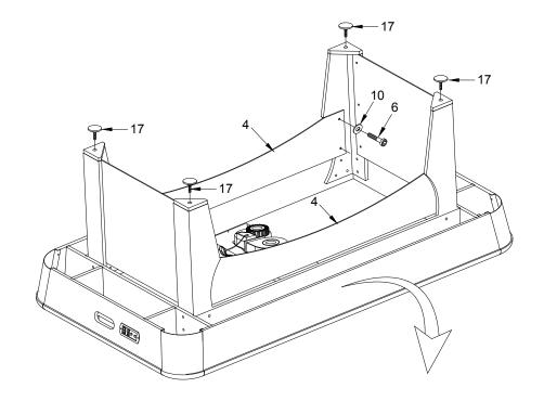
Attach Leg Connector (#4) to legs as shown, using four  $1/4 \times 3/4$ " Bolts (#6) and 1/4" Washers (#10).
