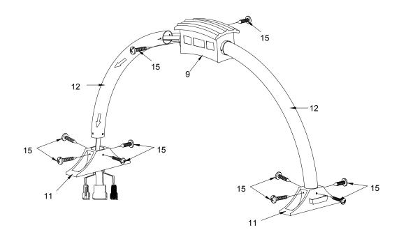
Thread Scorer cord through Scorer Support (#12) as shown. Attach Scorer Support to Scorer(#9) with 3 mm Screw(#15). Repeat on other side
