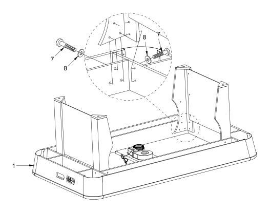
. Attach one leg/panel construction to Main Cabinet (#1), using 5/16" Bolts (#7) and 5/16" Washers (#8).
