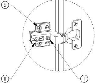
Tighten the Screw marked (I) to fasten hinge. The door may need to be adjusted so that all the spaces between the door and the unit sides are equal. To adjust, follow instructions:
