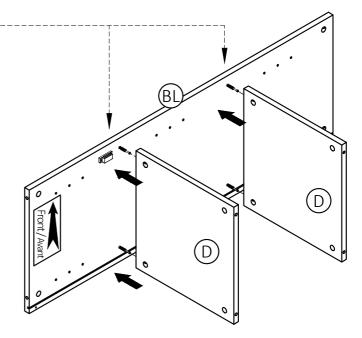
1. Align Cam Lock Pins with guide holes on parts ① and attach parts (D) to Left Side (BL).
