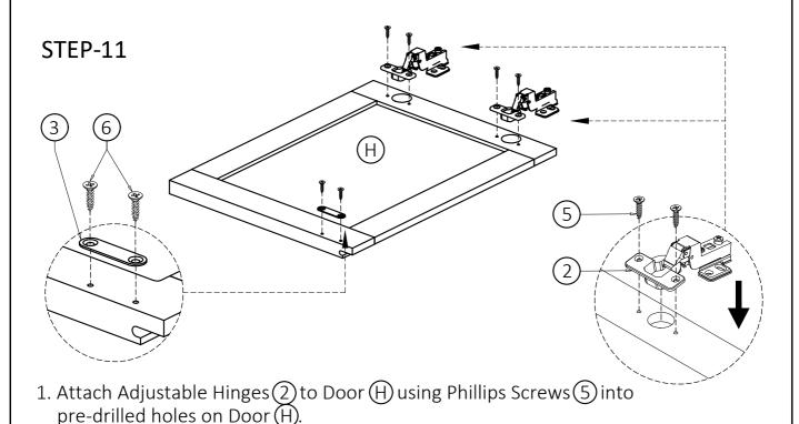
2. Attach Magnet Plate(3) to top corner of Door(H) using Phillips Screws(6) into pre-drilled holes on Door(H).
