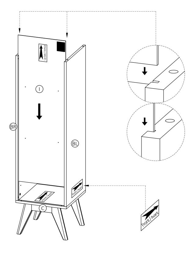
1. Slide Back Panel () firmly into slots on Sides (BL), (BR) and Bottom Shelf (C).
