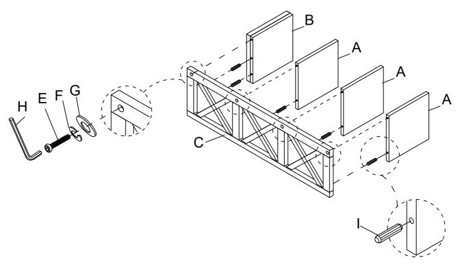
Attach Wood Dowel (I) to Side Panel (C) and Back Panel (D), then using Bolt (E), Lock Washer (F) and Flat Washer (G) to tighten Shelf (A) & Bottom (B) with Side Panel (C) & Back Panel (D) by Allen Key (H).
