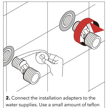
tape to ensure a watertight seal.
