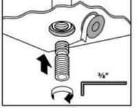
Rough-in: install a 1/2" NPT female fitting, recessed 3/8" inside the surface of the finished ceiling.
