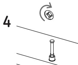
After joining two panels together you should turn the cams 180° with a phillips head screwdriver to adjust and secure the joint.
