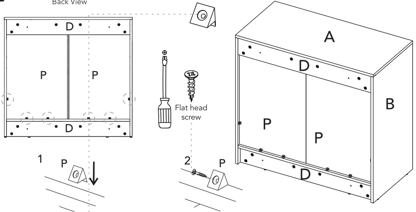
1 Insert the back panel supports between the groove and the back panel.
