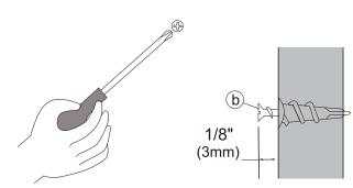
**Stud Mounting**(1b)Using a stud finder, locate and carefully mark the location of studs on the wall where you want to hang your shelf. Note: It is best to mount the shelf to at least one stud.
