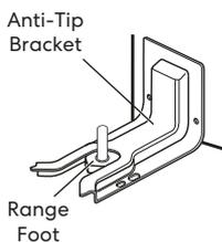
Making sure the anti-tip bracket is installed:
