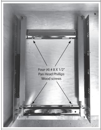
Place the slide base inside the cabinet, pulling the front cross member tight against the rear of the face frame. For frameless cabinets, set the front cross member back 3/4". For inset door applications, slide the base back from the above measurements plus the thickness of the door. Firmly secure with four (4) # 8 X 1/2" Pan Head Phillips Wood screws provided in the locations shown above.
