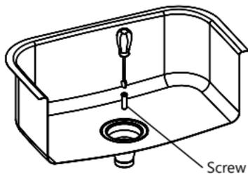
Using the screw, tighten the metal strainer and main body into place
