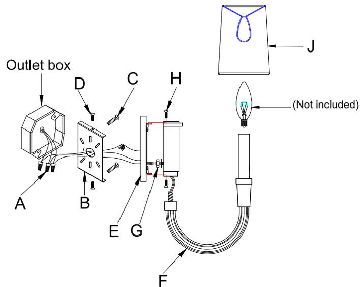
1. Remove plate (E) by unthreading screws (H) from the fixture.
