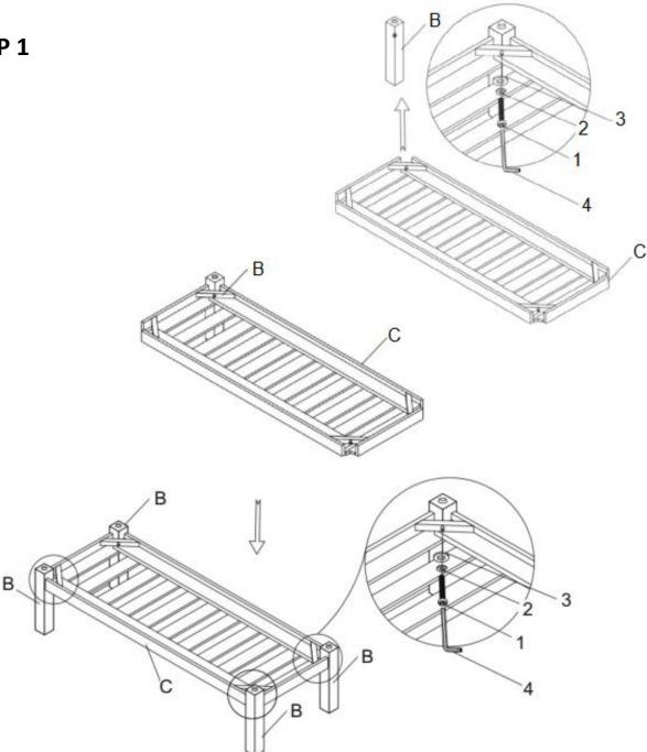
Attach Legs (B) to corners of Shelf (C) with Bolt (1), Lock Washer (2) and Flat Washer (3).
