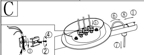
Always keep the fiberglass sleeving between the metal strain relief and the cord to protect the cord from damage
