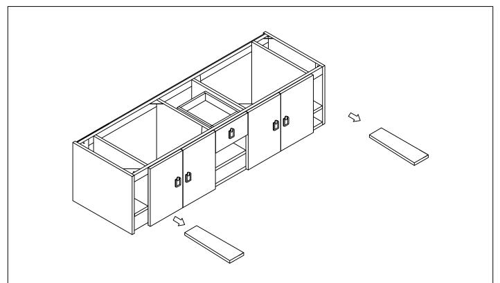
Step 3: Remove the shelves from top row for easier access to assemble the top.
