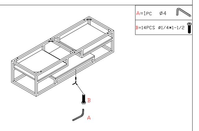
Step 2: Insert the bolt (B) from underneath of frame by using with Allen Wrench
