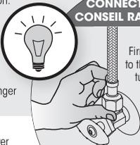
Firmly hand tighten the hose to the valve and add a quarter-turn using the proper wrench. Tighten more if needed.
