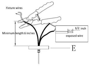
6 » Carefully pass supply wires through mounting plate assembly (A).
