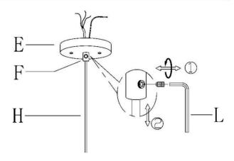
5 » If needed, shorten the extra length of the fixture wires from cord (H) so that they all are at least 6 inches (152.4 mm) long above canopy (E) within the outlet box.
