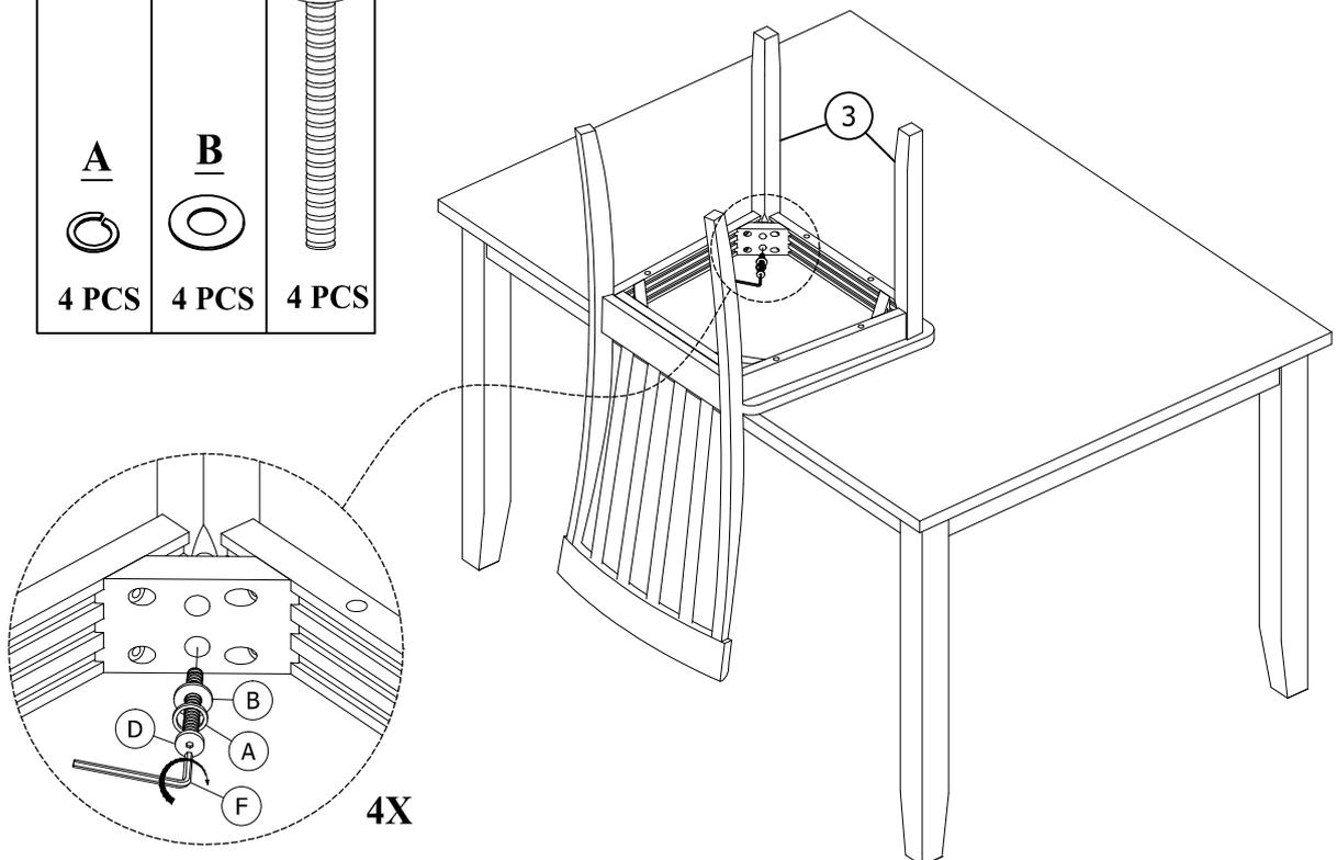
TIGHTEN BOLT COMPLETELY.
