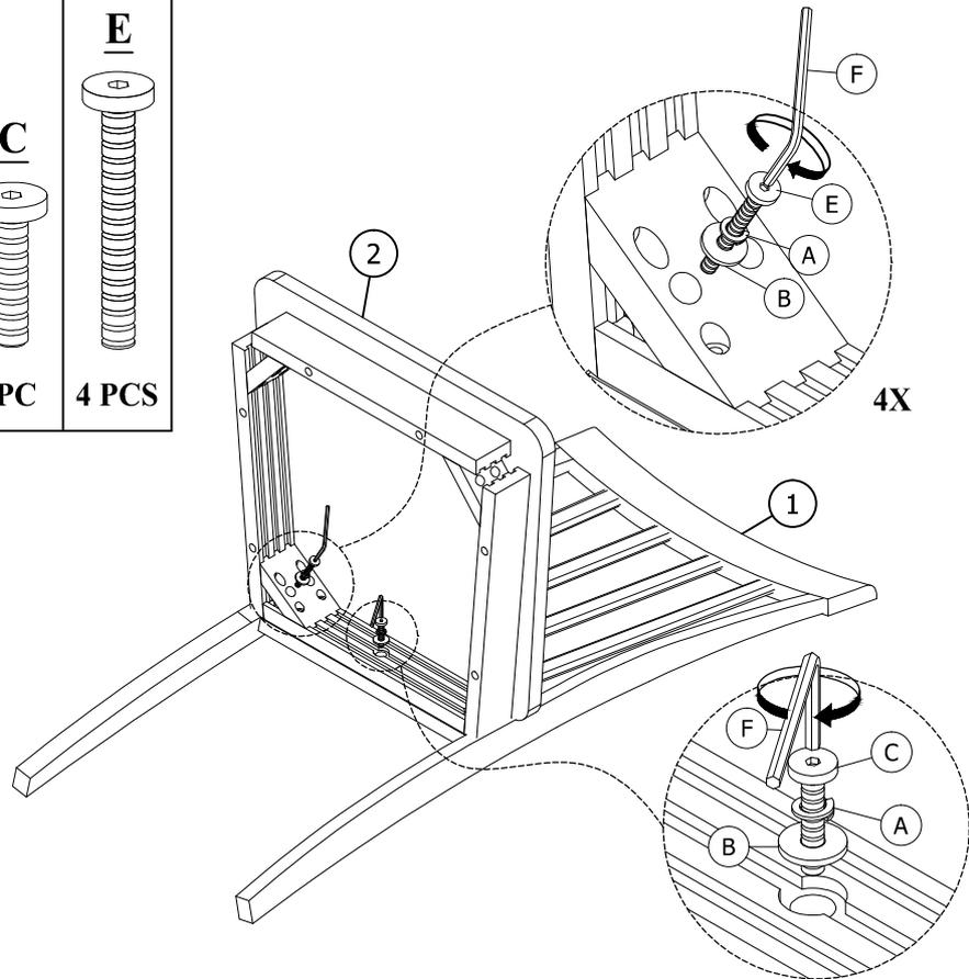
TIGHTEN BOLT COMPLETELY.
