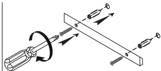
**IMPORTANT:** Consult an expert for the proper screws/bolts to use when attaching to various constructions. Screws provided do not attach to all wall construction types. Anchors are not required if brackets are installed in stud.
