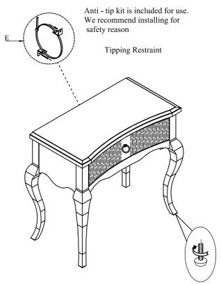
Adjust levelers if needed, to level case on uneven floor
