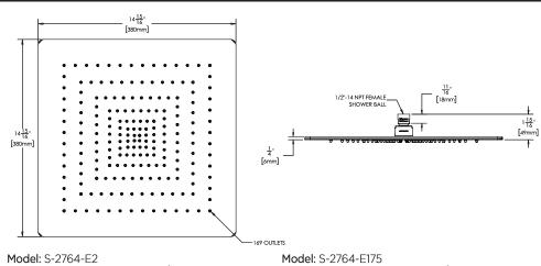
Max. Flow Rate: 2.0 gpm (7.6 L/min)
