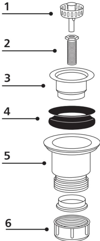
1. Apply a small bead of 100% Silicone (non-water based) to the underside of strainer body flange (3).
