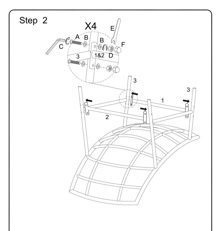
Attach parts (1,2) to part (3) using bolt (A), flat (B) and hex nut (D) with hex key (C) and open spanner (E). Then place screwdriver cap (F) on hex nut (D) per diagram.
