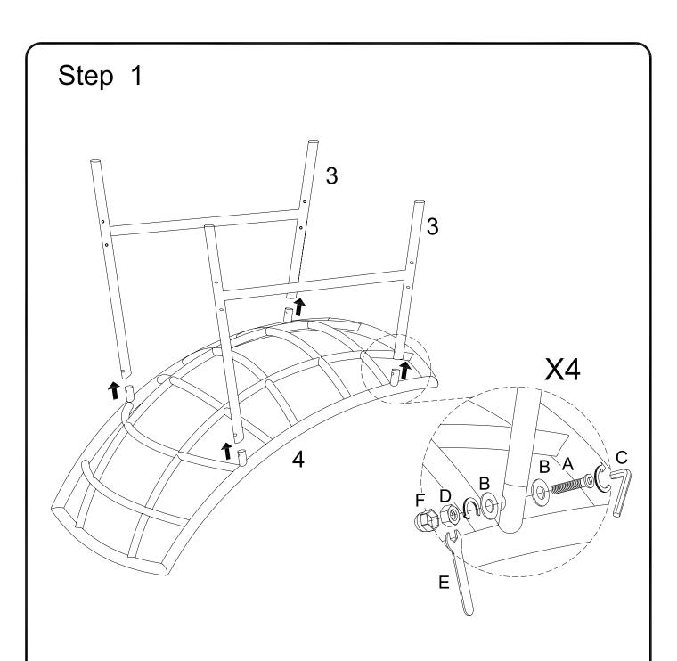
Attach part (3) to part (4) using bolt (A), flat (B), and hex nut (D) with hex key (C) and open spanner (E). Then place screwdriver cap (F) on hex nut (D) per diagram.
