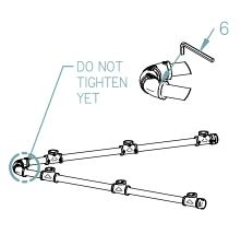
Make any necessary adjustments using 6 to loosen, adjust, and retighten any fitting.
