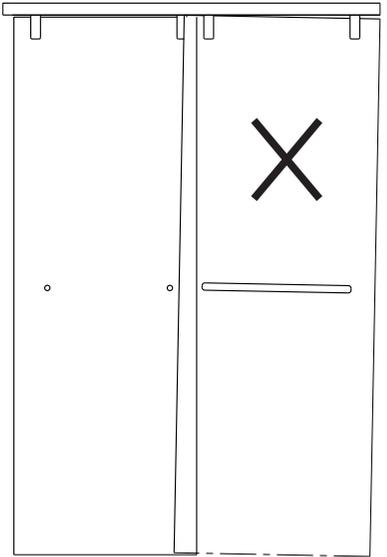
If the glass is in a slanting position after installation, it could be adjusted by the adjusting key , to make sure the glass is to be vertical.
