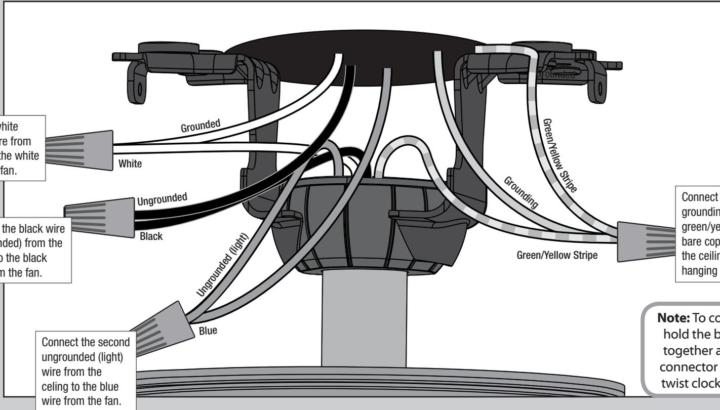
**Note:** To connect the wires, hold the bare metal leads together and place a wire connector over them, then twist clockwise until tight.
