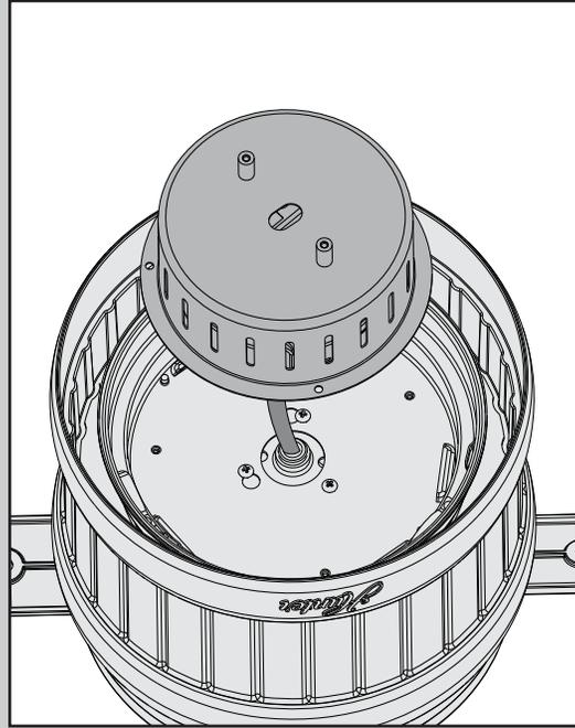
Lower the light kit. Align the screw holes in the light kit with the screw holes in the upper switch housing.
