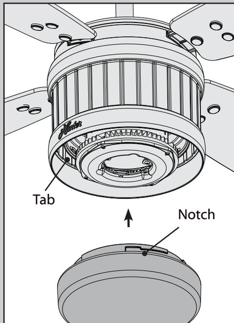
Position the notches in the outer rim of the globe so they line up with the tabs on the light kit assembly.
