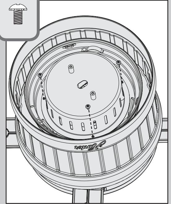
Install the three switch housing screws, found in the
