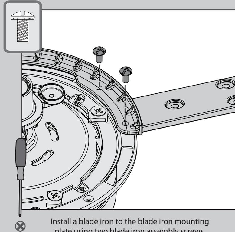
Install a blade iron to the blade iron mounting plate using two blade iron assembly screws, found in the X hardware bag. Repeat this process to install all blade irons.
