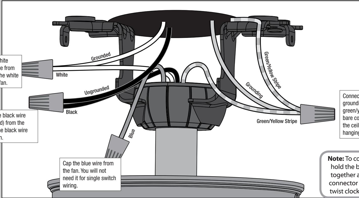
**Note:** To connect the wires, hold the bare metal leads together and place a wire connector over them, then twist clockwise until tight.
