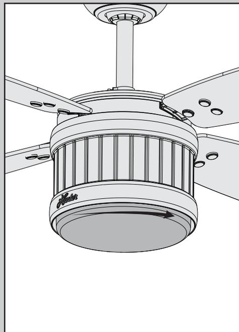
Carefully lift the globe up inside the light fixture as far as it will go. Rotate the globe in a clockwise direction until it is held tightly in place by the three tabs.
