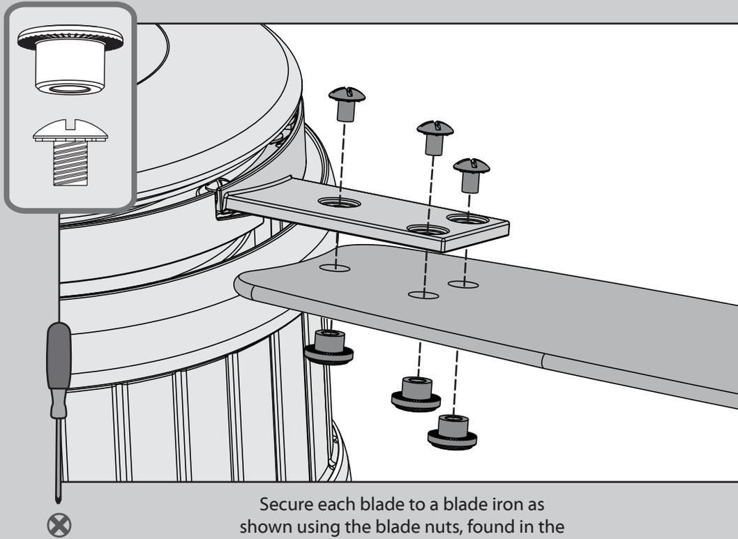
Secure each blade to a blade iron as shown using the blade nuts, found in the ■ hardware bag, and the blade assembly screws, found in the ▲ hardware bag.
