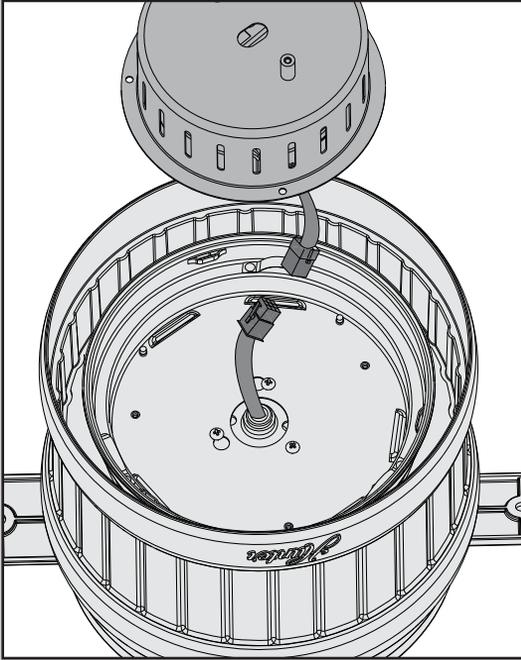
Connect the plug connectors found in the switch housing area of the light kit assembly. Make sure to line up the colored markings on the connectors.
