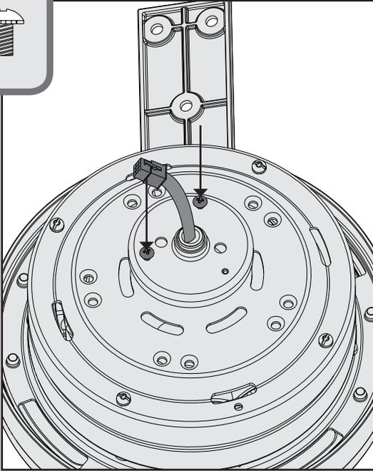
Partially install two light kit assembly screws, found in the ☰ hardware bag, halfway into the motor housing as shown. It does not matter which two screw holes you choose.
