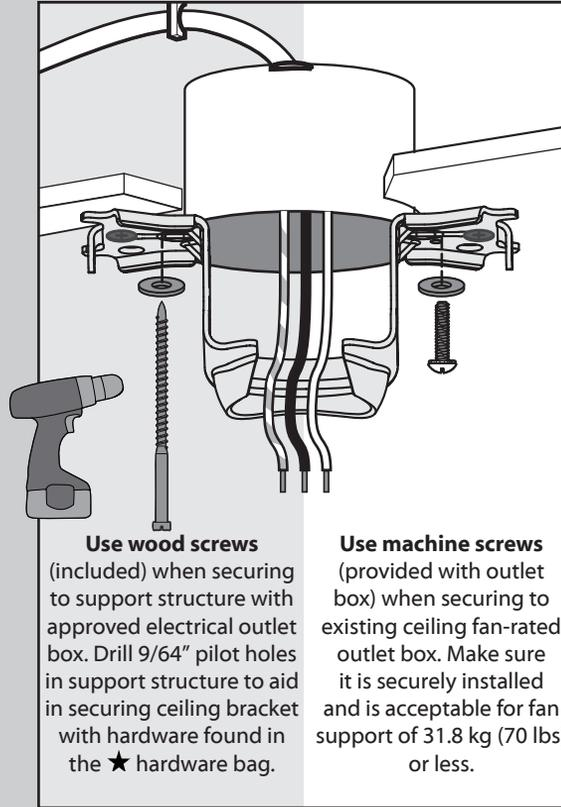
**Use wood screws** (included) when securing to support structure with approved electrical outlet box. Drill 9/64" pilot holes in support structure to aid in securing ceiling bracket with hardware found in the ★ hardware bag.
