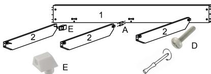
Fit the slat supports to the side rail, using the screws 4MA
