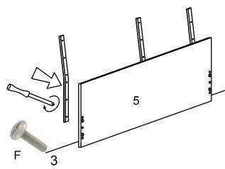
Fit the iron bars first on the under headboard and then on the hearboard, using the screws 6MA
