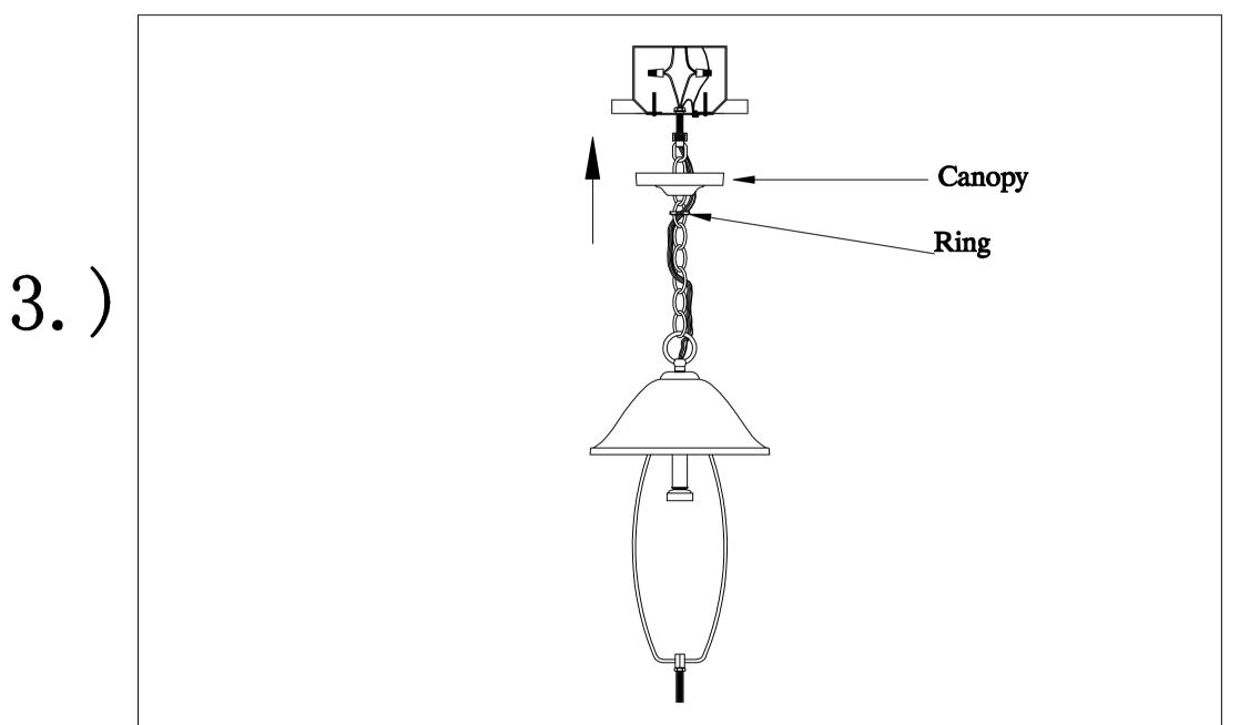
Step.3: Remove ring from loop and slide down chain. Place canopy onto chain and let slide to top of fixture. Install screw collar loop to bracket. Pull canopy through screw ring up chain to ceiling and tighten securely.
