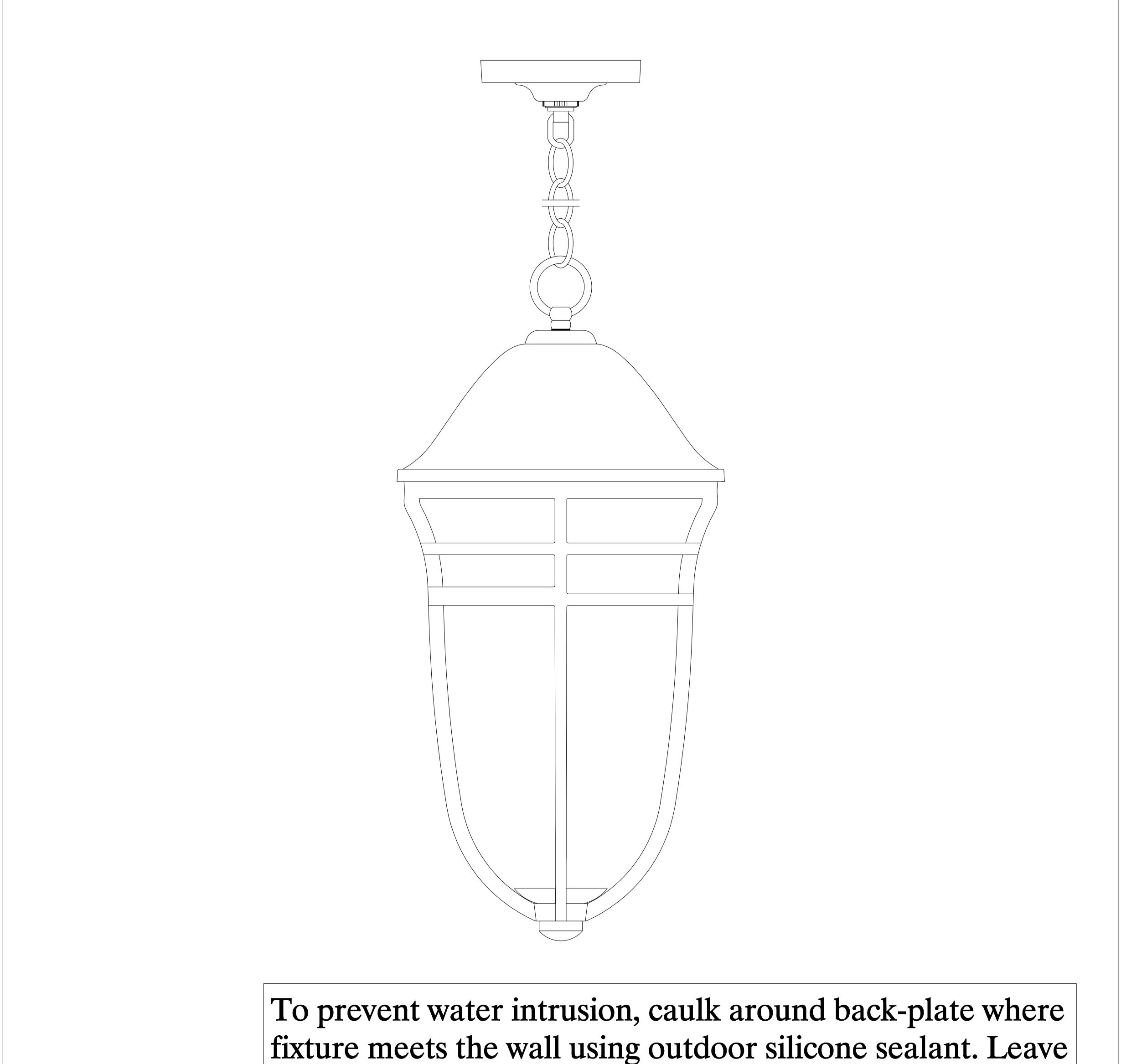
fixture meets the wall using outdoor silicone sealant. Leave a small gap at the bottom to allow moisture to exit.
