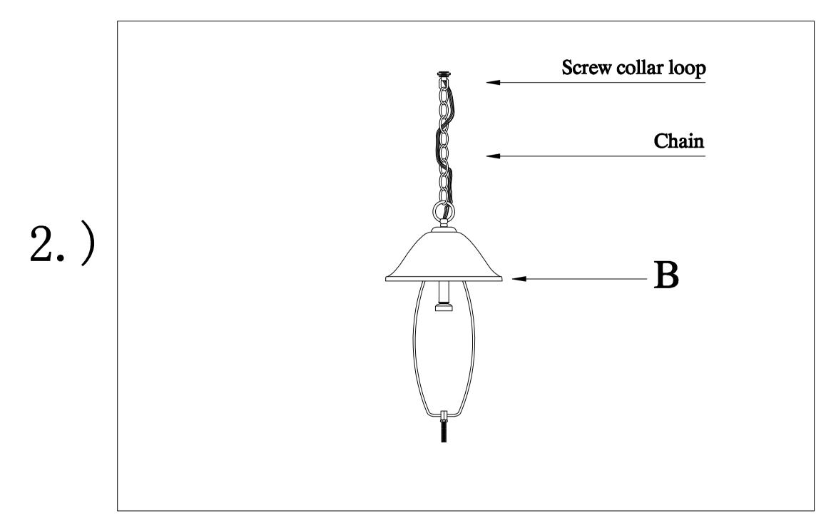
Step.2: Install chain to fixture(B), install screw collar loop to chain. Attach appropriate amount of chain to loop to achieve desired mounting height. Thread wire through every 3rd loop of chain.
