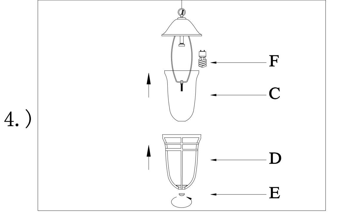
Step.4: Install GU24 bulb(F), attach glass(C) and cage(D) and finial(E).
