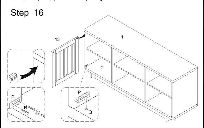
Place door hinge (P) into plastic pivot (Q) on part (2). Insert top door hinge into plastic pivot (Q) on part (1), then slide the door (13) into the bottom hinge (P). Secure door by tightening door hinge (P) using screws (R) with equal pressure.
