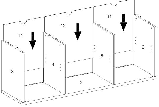
Slide back panel (11,12) into grooves as per diagram.
