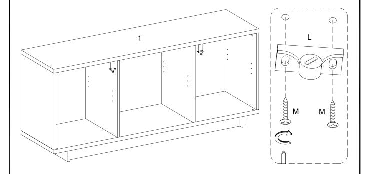
Attach door stopper (L) to part (1) using bolt (M) with screwdriver.
