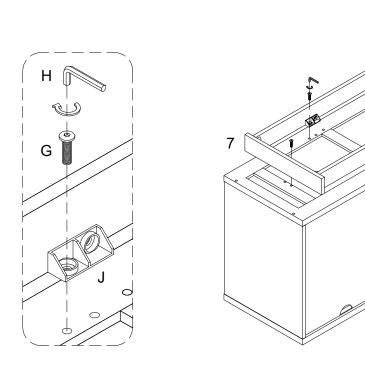
Attach connector (J) to part (2) using bolt (G) with hex key (H).
