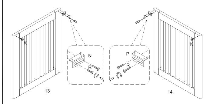
Attach door hinge (N,P) to part (13,14) using screw (R) with screwdriver. Attach bolt (K) to part (13,14) with screwdriver.
