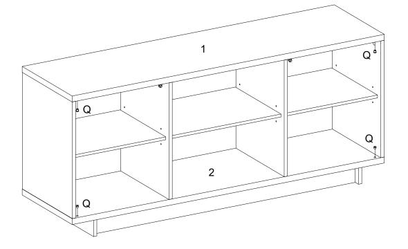
Place plastic pivot (Q) over holes as per diagram.
