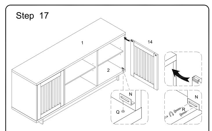
Place door hinge (N) into plastic pivot (Q) on part (2). Insert top door hinge into plastic pivot (Q) on part (1), then slide the door (14) into the bottom hinge (N). Secure door by tightening door hinge (N) using screws (R) with equal pressure.
