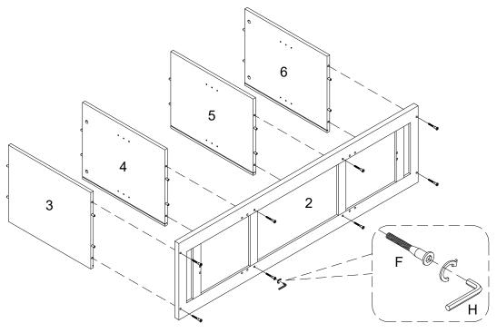
Attach part (2) to part (3,4,5,6) using bolt (F) with hex key (H).
