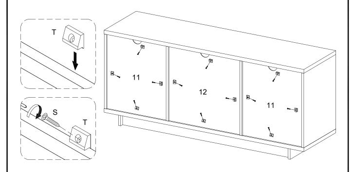
Attach plastic wedge (T) to part (11,12) using screw (S) with screwdriver.
