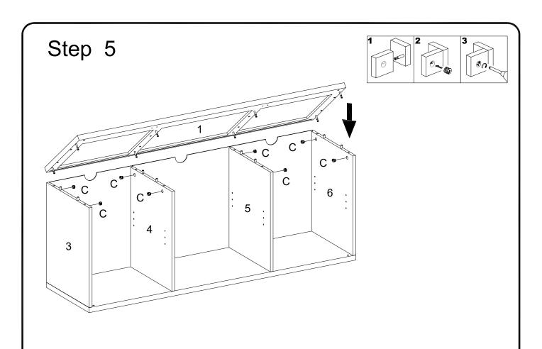
Attach part (1) to part (3,4,5,6), then insert and secure cam lock (C) to part (3,4,5,6) to lock it.
