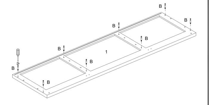
Attach cam bolt (B) to part (1) with screwdriver.
