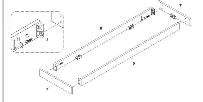
Attach connector (J) to part (7) using bolt (G) with hex key (H).
