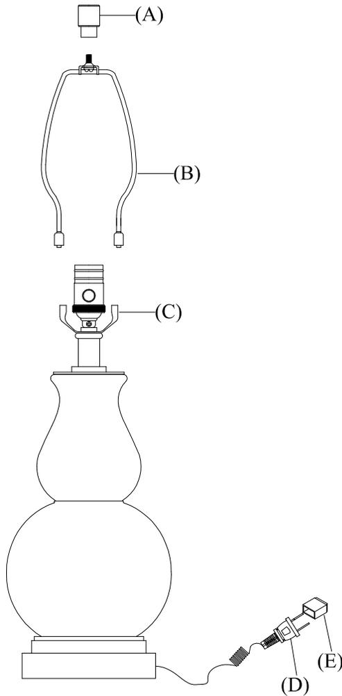
1. Insert harp (B) into harp saddle (C) by squeezing both sides of the harp.
