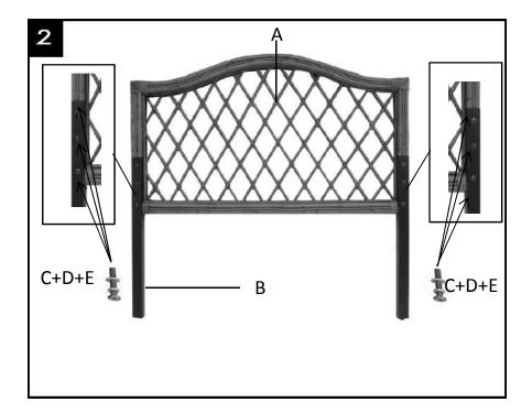
Step 2 Attach the two legs (B) to the headboard (A) using 6 bolts (C), 6 washers and 6 rings. Others 6 bolts, washers and rings are attached on the legs.
