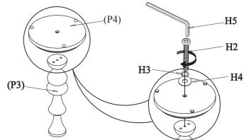
Step 2. Attach the Mounting Plate (P2) to Post (P3) as shown below.
