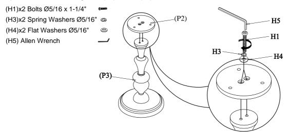
Step 3. Attach the Mounting Plate (P2) to Table Top (P1) as shown below.
